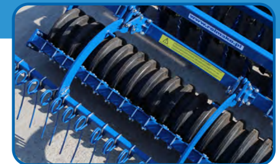
Rubber roller Ø 500 mm
