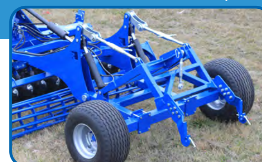
Drawbar + trailer with a seeder coupler
