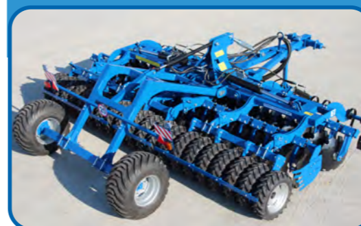
Trailed disc harrow with a tire roller
