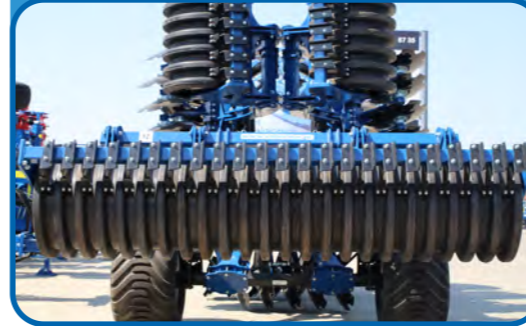
Prismatic roller ORION Ø 500 mm
