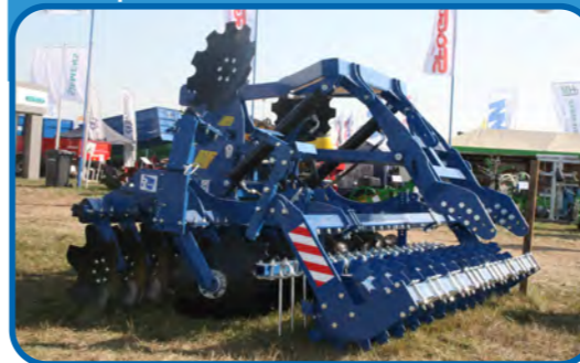
Trailed disc harrow with a tire roller
