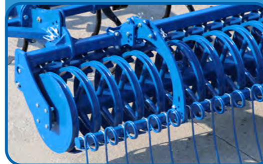
Steel ring roller Ø 600 mm
